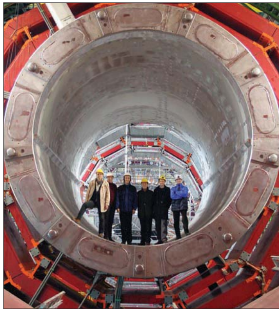
Fig. 1. Members of the CMS Magnet and Integration Group and representatives from Saclay stand inside the cryostat of the giant superconducting solenoid during cooling to the interior operating temperature of 4.5 K.
