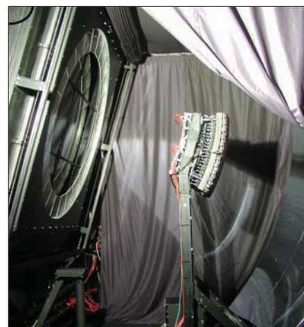
Fig. 4. The 440-photomultiplier camera at one of the fluorescence stations.
