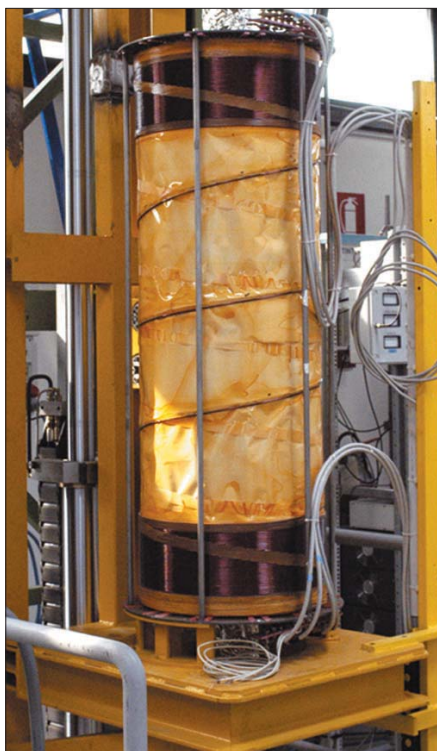
Detail of SAES' sputtering system used to apply the IntegraTorr coating, capable of processing up to seven-meter long chambers.
