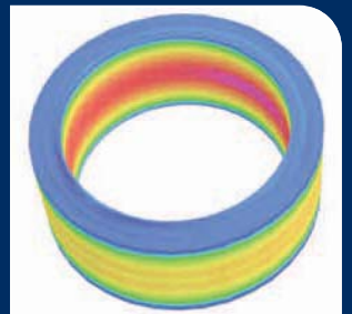
Propagation of a quench in a superconducting magnet
