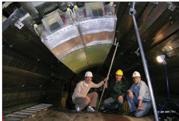
Fig. 3. The first two supermodules of the ECAL were installed into the barrel of the HCAL with the help of the CMS ECAL Group, CMS Integration and CEA-DAPNIA.
