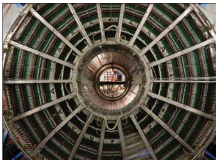
The ALICE TPC in its clean room, where it is undergoing commissioning of all its sectors.
